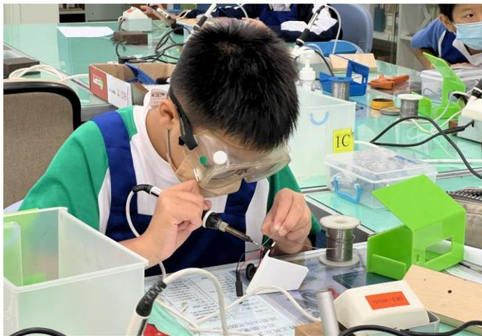
銲接,並以熱縮膠管套銲接位作絕緣
