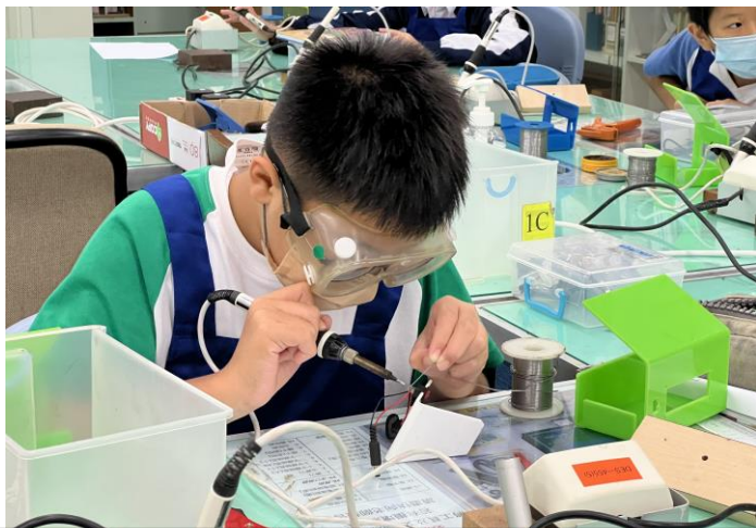
銲接,並以熱縮膠管套銲接位作絕緣
